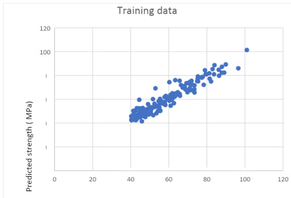
Fig. 9 – Graph for Actual versus Predicted compressive strength by DNN for training data
